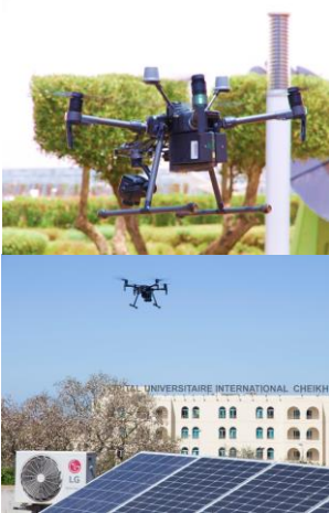
RGB and thermal infrared on-field image acquisition
